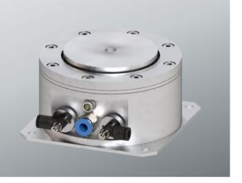
Low-frequency diaphragm air spring with integrated electro-pneumatic level control for effective vibration isolation and decoupling of highly sensitive equipment and processes.
